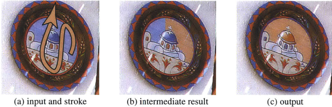
Figure 3-5: Bilateral Grid Painting allows the user to paint without bleeding across image edges. The user clicks on the input (a) and strokes the mouse. The intermediate (b) and final (c) results are shown. The entire 2 megapixel image is updated at 60 Hz. Memory usage was about 1.5 MB for a 20 \times 20 brush and s_r = 0.05 .
