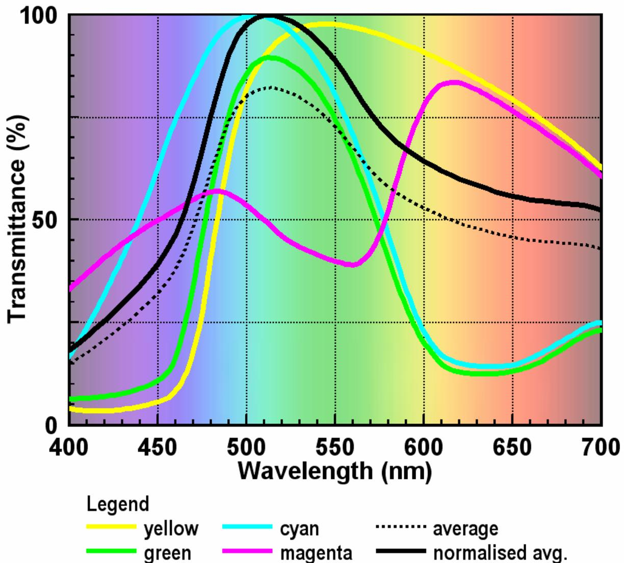
Figure 1 Spectral Response Of The Sony ICX418AKL-A CCD
