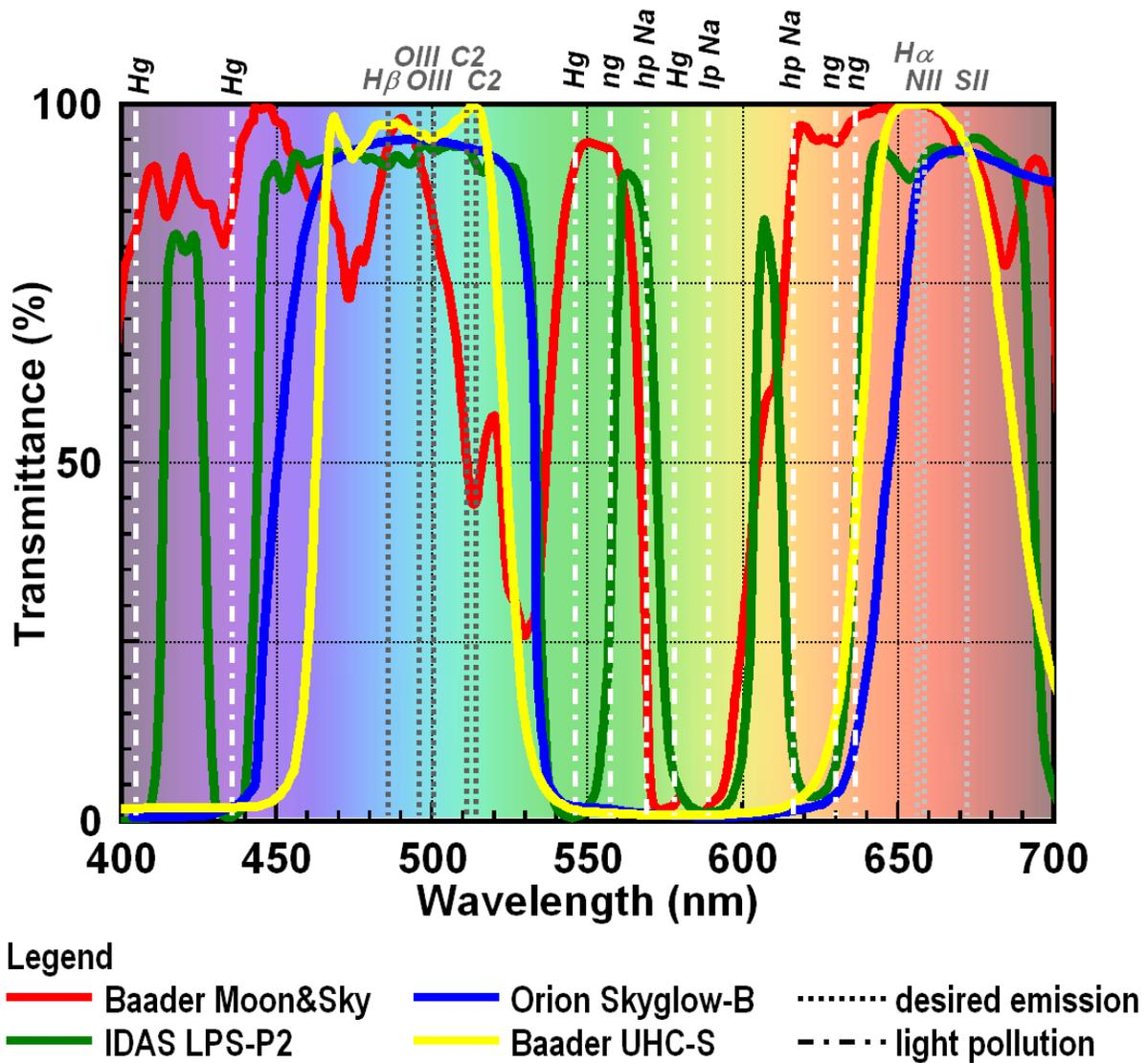
Figure 4 Band-Pass Filters Used In Test - Part 1
