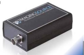
HD-SDI is a serial, digital interface, primarily designed to transmit uncompressed and unencrypted video data over one or more coaxial cables with BNC connectors at a nominal impedance of 75 ohms. The cabling and connector type are relics from the previous analog video signal standard. When using high quality cable, the maximum cable length can be up to 100 meters.
