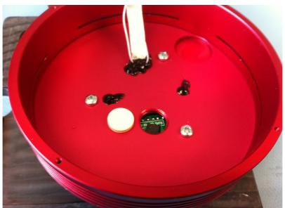
Once removed the tablet can be replaced with new or baked in an oven at 200 degrees Celsius for around 60 to 90 minutes, this will regenerate the tablet.
