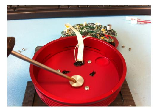
Once removed the desiccant tablet is visible, invert the camera carefully and allow the tablet to fall out.
