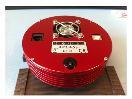
Locate the silver or black plug of the desiccant chamber and remove by unscrewing anti clockwise. You may need to use pliers to assist with this.
