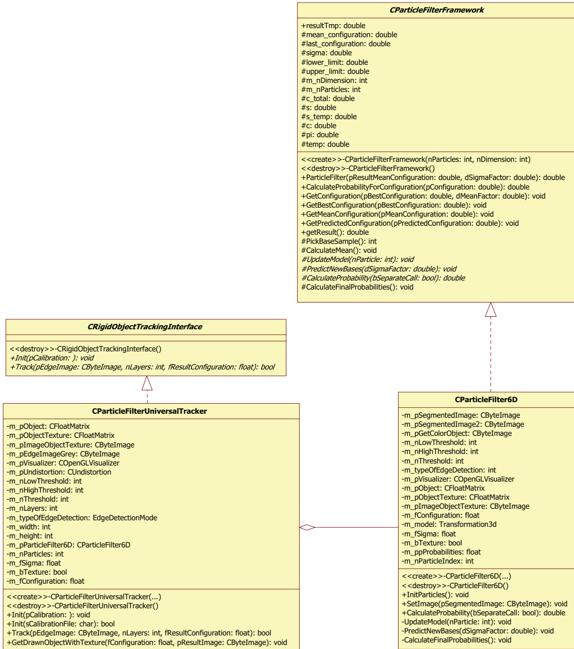
Figure 5.1: UML class diagram of the implemented approach.
