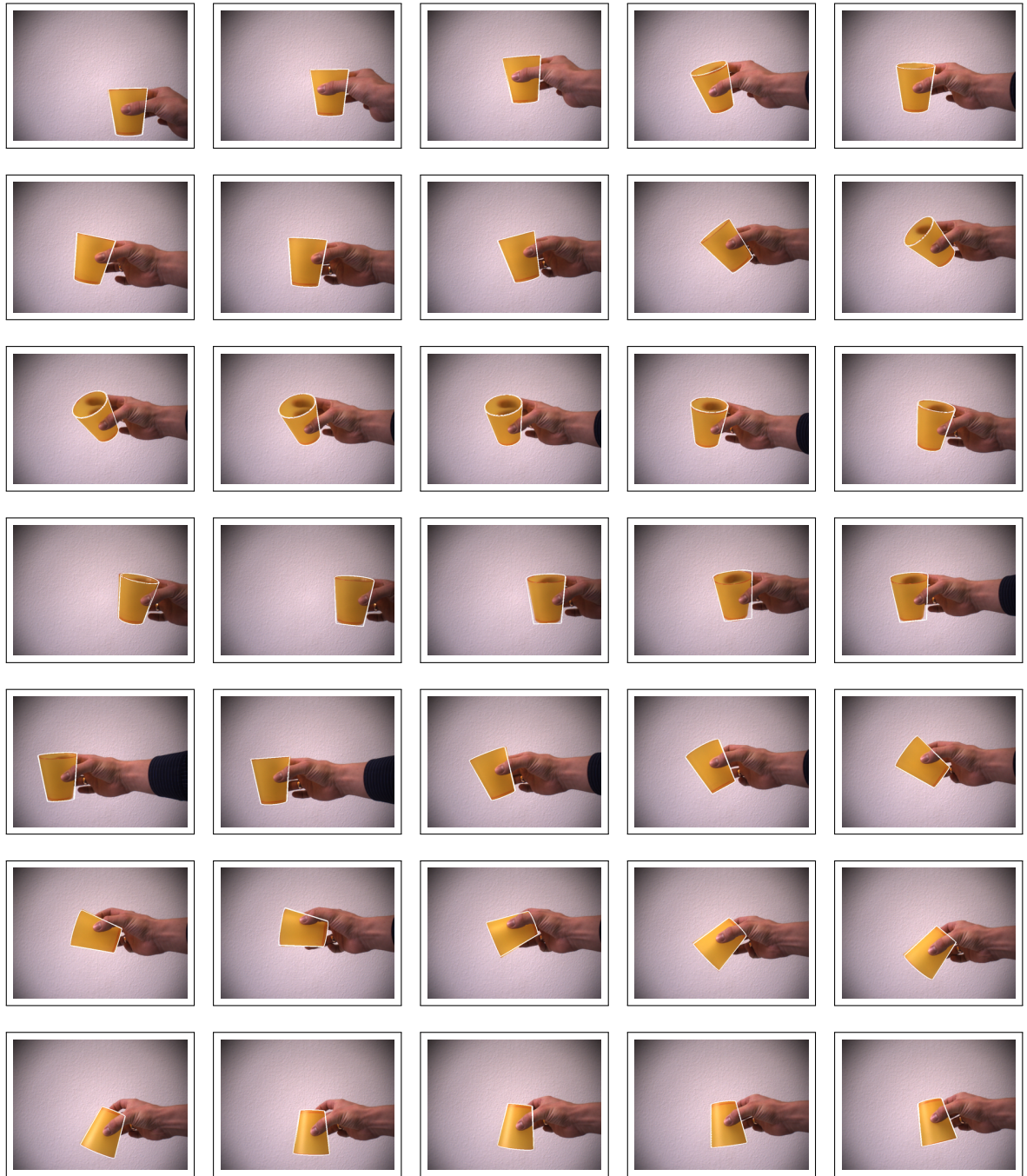
Figure 6.19: Tracking of a yellow single-colored cup. Parameters: Every fifteenth frame of a sequence of 525 frames is shown. The Sobel operator was used and an amount of 500 particles per layer, with a total of 5 layers. The initial configuration is x = 57\text{ mm} , y = 61\text{ mm} , z = 480\text{ mm} , \alpha = 0^\circ , \beta = 1^\circ and \gamma = -1^\circ . The variance is 5\text{ mm} for translation and 4^\circ for rotation.
