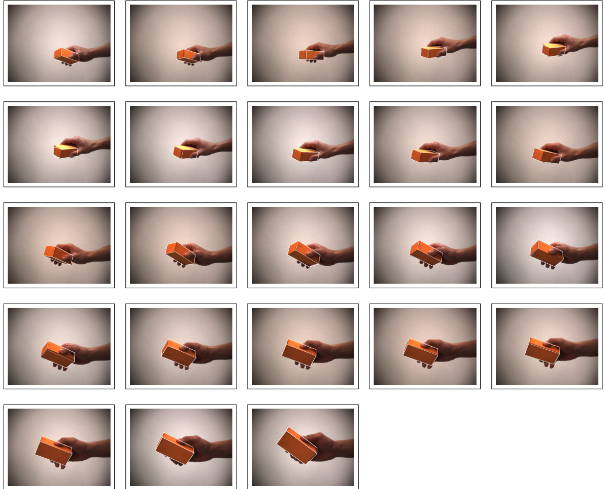
Figure 6.21: Tracking of an orange single-colored cuboid. Parameters: Every tenth frame of a sequence of 230 frames is shown. The Sobel operator was used and an amount of 250 particles per layer, with a total of 6 layers. The initial configuration is x = 36\text{ mm}, y = 37\text{ mm}, z = 676\text{ mm}, \alpha = 60^\circ, \beta = -23^\circ and \gamma = 37^\circ . The variance is 5\text{ mm} for translation and 2^\circ for rotation.
