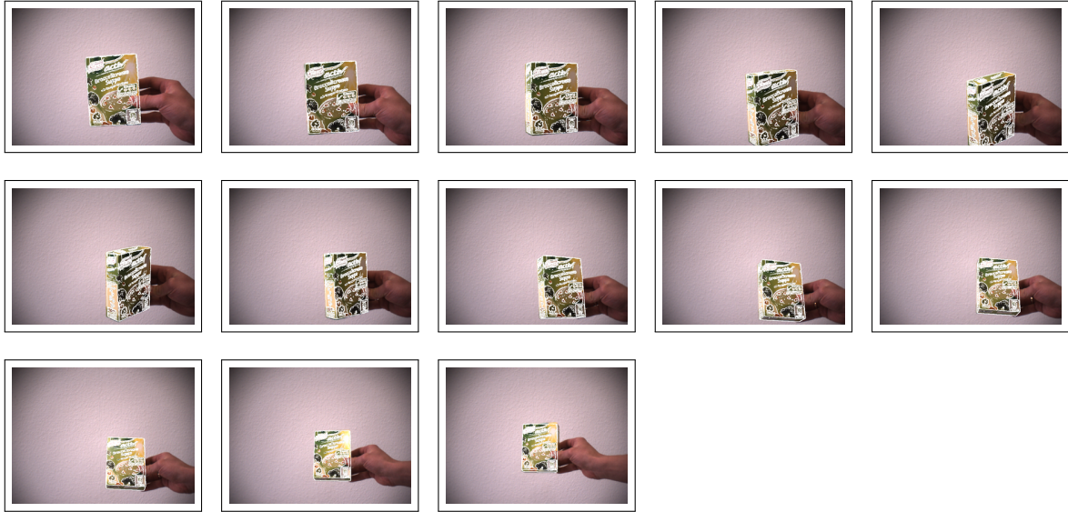
Figure 6.23: Tracking of a colorful textured box of soup. Parameters: Every tenth frame of a sequence of 130 frames is shown. The Sobel operator was used and an amount of 1000 particles per layer, with a total of 10 layers. The initial configuration is x = 21\text{ mm} , y = 32\text{ mm} , z = 492\text{ mm} , \alpha = 80^\circ , \beta = 54^\circ and \gamma = -57^\circ . The variance is 5\text{ mm} for translation and 2^\circ for rotation.
