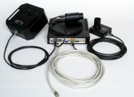
The Ethernet interface supports transmission speed 1 Gbps and slower 10/100 Mbps and allows integration to all common local area networks. Compact unit uses the same supply voltage 12 V DC and power connectors like G2, G3 and G4 cameras. Thus, it is possible to use the identical power source for the ETH Adapter as for the rest of system.
