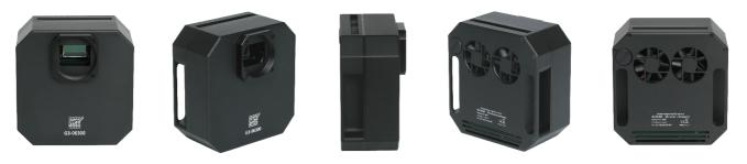
G3 cameras can be equipped with CCD detectors up to  $24 \times 36$  mm. Precisely regulated and efficient cooling of the CCD up to  $45^{\circ}$ C below ambient temperature allows quality image calibration. There are mechanical shutter and filter wheel with 5 positions for 2-inch (or 50 mm) round filters inside the camera head, so these cameras can be used in unattended, robotic setups. G3 cameras can be also combined with external filter wheels with 7 positions for 2-inch (or 50 mm) filters.
