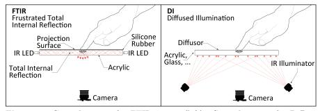
Figure 2. General set-up of a FTIR system (left). General set-up of a Diffuse Illumination system (right). The projector is mounted inline with the projector below/behind the surface.
