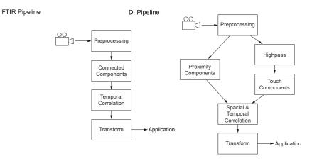
Figure 5. FTIR Tracking Pipeline (left). DI Tracking Pipeline (right).
