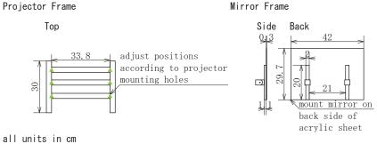
Figure 6. Detailed engineering drawing for an interactive multi-touch table.
