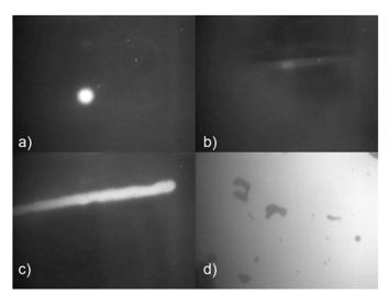
**Figure 4.** (a) Rigid PVC (backlit) (b) Rosco translucent [4] (c) Sihl polyester film 100 at, and (d) HP backlit UV. Using the wrong combination of materials can results in two main problems: (b) either the FTIR effect is not strong enough; or (d) the layers stick together.
