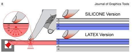
Figure 3. The three layers needed to track the finger touches: the polycarbonate plate (a) is covered with a compliant surface layer (b) and a diffuse layer (c) on top (left). Silicone compliant layer: the gap (c) is between the projection surface (d) and the combined silicone (b) polycarbonate (a) layer (right top). Latex compliant layer: the projection (d) and the latex layer (c) must be combined; the gap (b) is between these two and the polycarbonate plate (right bottom).
