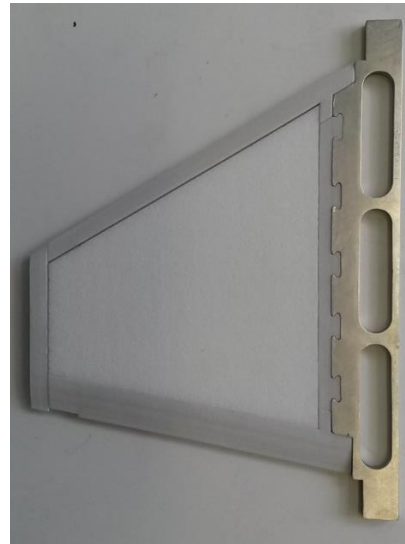
Figure 26. Additive manufactured frame with aluminum backbone and foam core
