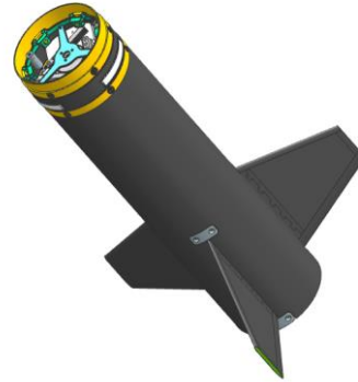
Figure 34. Control System above the Motor Section
