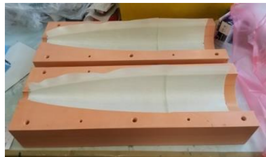
Figure 9. GFRP prepreg sheets draped in half shell molds
