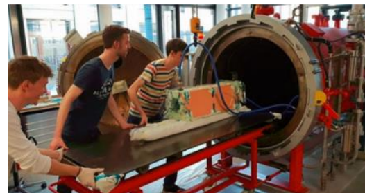
Figure 12. Vacuum bagged mold is moved in the autoclave
