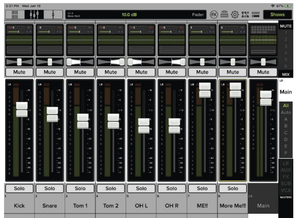
Mackie's Master Fader, one of many manufacturer apps that offer tablet mixing of FOH or multiple monitor feeds. This particular example shows a commonly encountered performer mix featuring two maxed-out channels providing "me" and "more me."
