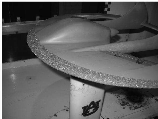
Fig. 3 Geobat model with transition strip installed in the wind tunnel.
