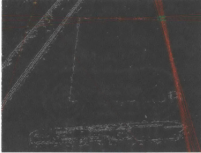
Figure 3-12: Example of a Cluttered Writing Surface. Our page detection algorithm will fail for this video frame because it contains too many objects that distract away from the actual page. The frame is shown after the Canny edge detection and Hough line detection steps to show the effects of the interfering edges. In the top-left corner of the video frame is a ruler and toward the bottom is a pen.
