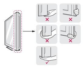
When holding the TV, the screen should face away from you to prevent the screen from scratches.
