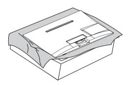
2 Attach the Stand Body from the TV. Insert the two Lockers of the Stand Body right into the groove of the TV head and secure them by pressing the left and right bottom sides.
