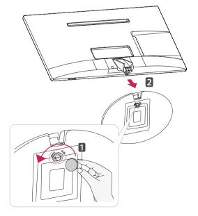
3 Remove 2 screws and pull out the Stand Body from the TV.
