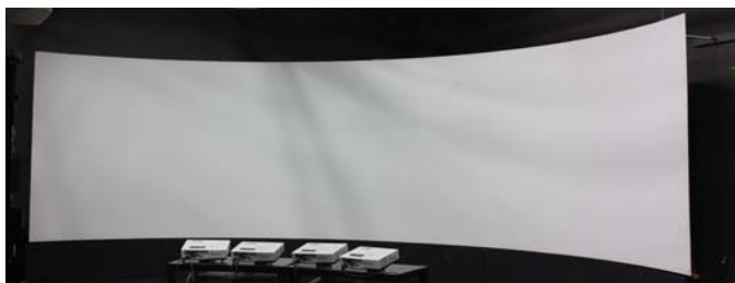
Fig. 5. The image used for calibrating a cylindrical display with 2 \times 4 array of eight projectors. This image of the screen, with no projectors turned on, used for recovering the camera and the display properties.
