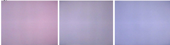
Figure 8. This figure demonstrates the white point emulation. The original non-standard reddish white (0.35,0.325) in CIE xy space (left) has been changed to a neutral D65 white (middle) and a bluish D85 white (right) using our white emulation.
