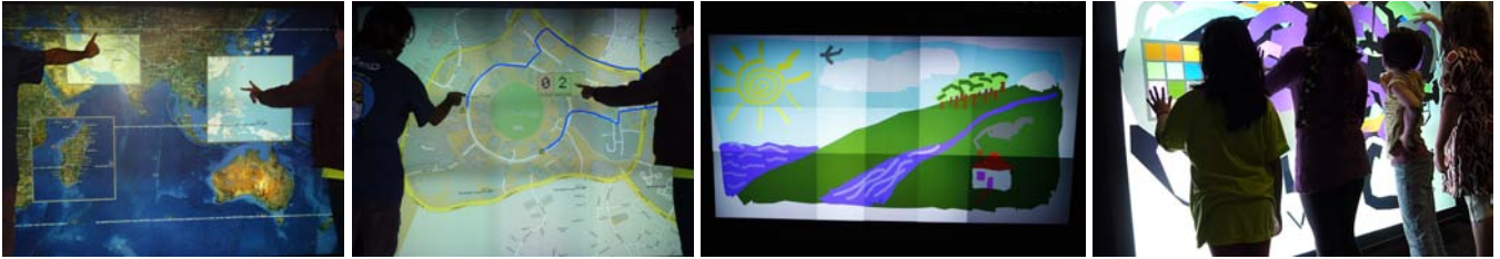
Fig. 1. This figure shows some of our applications in action. From left to right: Our collaborative map visualization application with two users visualizing different parts of the map at the same time on our 3 \times 3 array of nine projectors; Our collaborative emergency management application with two users trying to draw a path to hazardous location and dispatching teams of first responders on our 3 \times 3 array of nine projectors; Digital graffiti drawn using our collaborative graffiti application on only six of the projectors. We deliberately did not edge blend the projectors to show the six projectors clearly; Four children working together on our digital graffiti application on a 3 \times 3 array of nine projectors.
