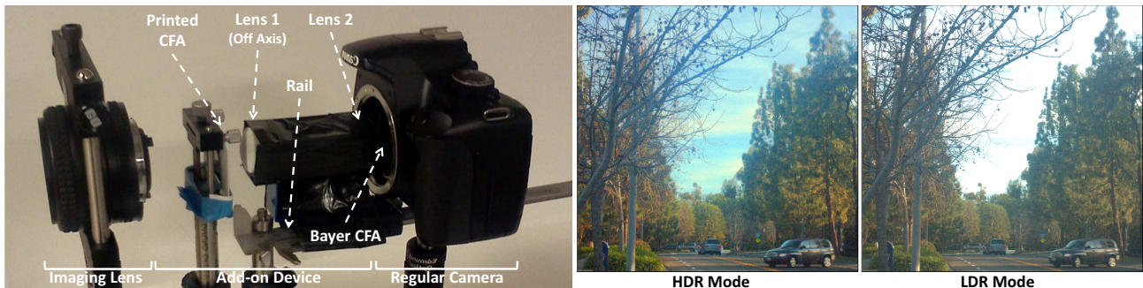
Figure 14: Left: This figure shows the design of the add-on device that be added to a regular Bayer LDR camera to achieve a HDR mode. A pair of lens, separated by a fixed distance, is put between the Bayer CFA on the camera sensor and the printed CFA. The lens which is close to the CFA is slightly off-axis. The amount of shift is controlled moving this two-lens ensemble on a rail. Right: We show the LDR and HDR images captured by this prototype. Note the saturated sky in the LDR mode is better captured in the HDR mode.
