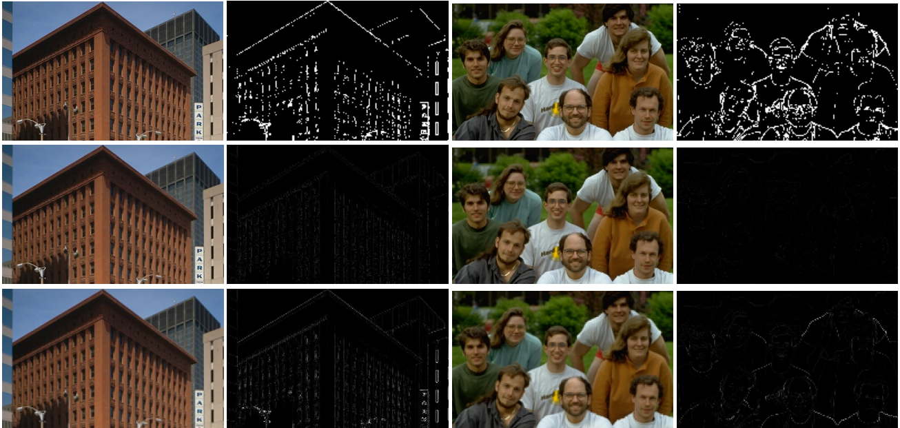
Figure 2: Columns 1 and 2 show the results on a BUILDING image, 3 and 4 show the results on a PEOPLE image ( c = 2 ). Top row: target high resolution image ( I ) and the chosen edge pixels. Bottom row: low resolution image I_l ; and its CIELAB \Delta E difference from I . Middle row: edge-enhanced image, I_v , i.e. the output of our system, created by superimposing I_e and I_{ne} ; and the CIELAB \Delta E of I_v from I . Compare the differences in the text 'PARK' and the lampposts in BUILDING and faces in PEOPLE in I_v and I_l . Please zoom in to see the differences.
