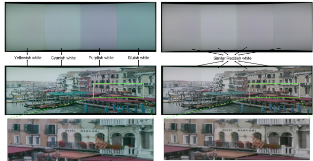
Figure 9. Please zoom in to see our curved screen display made of four projectors (real system, not simulated) running our color balancing algorithm. Top: This shows the whites before (left) and after (right) our color emulation matching to an NTSC gamut. Note that the brightness balancing across projectors described in Section 4.2 is still not applied. Hence, intensity variation and seams are still visible. Middle: This shows a regular content (Venice) before (left) and after (right) our color emulation for each projector to match the NTSC gamut, followed by our TTV (and hence brightness) balancing across projectors and finally removing spatial variation in TTV (and hence in brightness) using existing camera-based calibration methods. Bottom: In this zoomed in views, compare the colors of the buildings near the text Hotel Marconi to see the effect of our color balancing.
