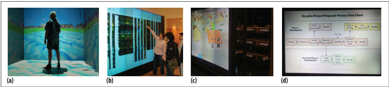
Figure 1. Early large area displays. (a) University of Illinois at Chicago's CAVE and (b) Princeton University's 18-megapixel display wall, which uses a 6 \times 4 array of 24 projectors. (c) UCI's 7-megapixel wall, which uses a 3 \times 3 array of nine rear projectors, showing (d) a completely seamless image that looks like a single projector display, although it comes from nine projectors. The UCI projectors had severe color variations, which researchers alleviated by developing camera-based automatic registration software.
