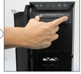
Slide your 5.25" drive through the front chassis until it lines up flush with the front bezel.
