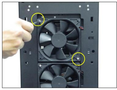
Be sure to screw in the fan in the top-left and lower-right holes first.
