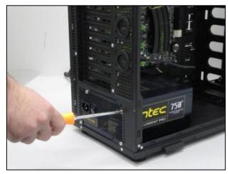
Attach the power supply with the provided screws.
