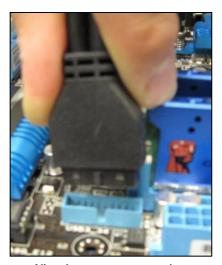
Align the connector properly to prevent damage to your motherboard.
