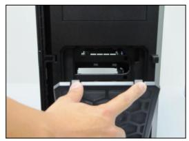
The P280 features a removable PSU filter that can be unlocked for maintenance and locked for transport. To remove the PSU filter, push the ends of the filter down then pull the filter toward you using the tab outside of the chassis. You can also lock the filter by pushing up on the tab (once the filter is completely inside the chassis).
