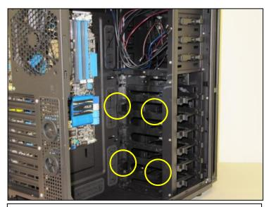
Align your fan with the pegs that correspond with the fan screw holes on the fan.
