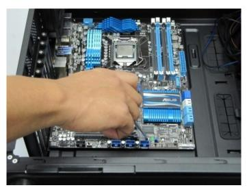
Use the provided motherboard mounting screws to secure your motherboard into the standoffs.
