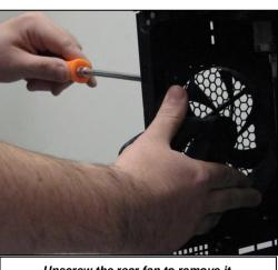
Unscrew the rear fan to remove it.
