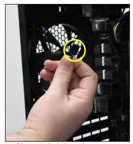
Disconnect the 3-pin power connector.
