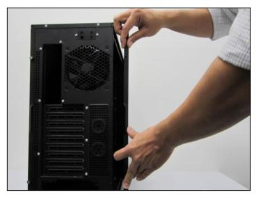
Remove the panel by the end of the panel at the top & bottom and swing the panel outward.
