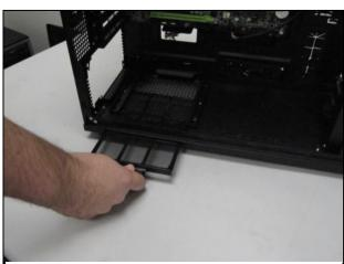
Remove the filter by pulling on the tab outside the chassis.
