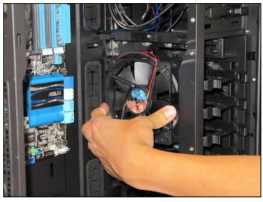
Secure an intake fan into place by aligning it with the pegs that correspond with the fan screw holes.
