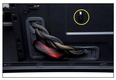
Use the grommet-lined cable routing holes to route PSU cables.
