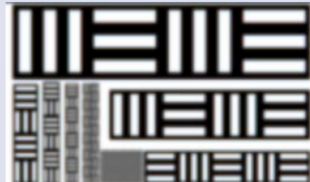
Resolv4K Zoom @ 4.5X High Mag 8.9MP Sensor - 0.76 \mu m / pixel 3.56mm FOV - 5.20 mm 2 Area (3.25X more)
