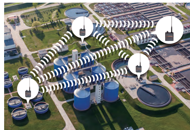
GW1-ETH-WQ-US Gateway terminal (master) for computer AI-1004LY-WQ-US Analog input terminal (slave) 10-bit, 4ch, ±10V DIO-0404LY-WQ-US Digital I/O Terminal (slave) isolated input 4ch, output 4ch
