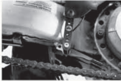
Fig. D Installation example on VFR750 (same method as 800) NB: longer 7 hole bracket. Oil can also be dispensed onto chain, above the inner side-plates, just in front of sprocket. If you have a 'hugger' fitted, you may find the spacer requirement differs from that shown. You must ensure that spacers used allow the body of the dual injector to lie in line with the chain.
