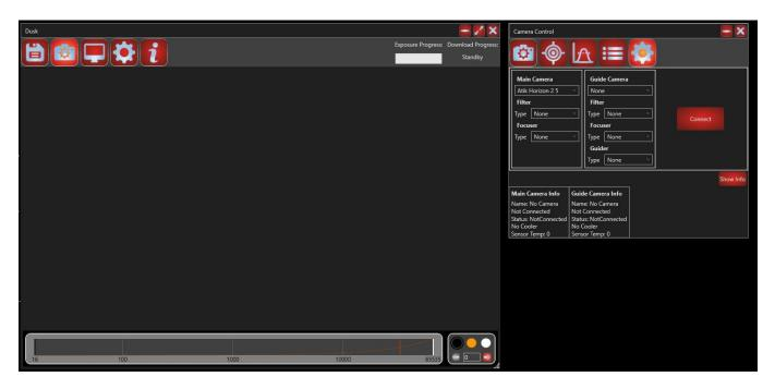
Upon opening Dusk, select the Setup icon , with the Horizon II connected to power and USB3 you should see the screen above. The Horizon II should be automatically found and be displayed as the main camera. If it isn't click on the box drop down symbol and select the camera and connect to the camera.
