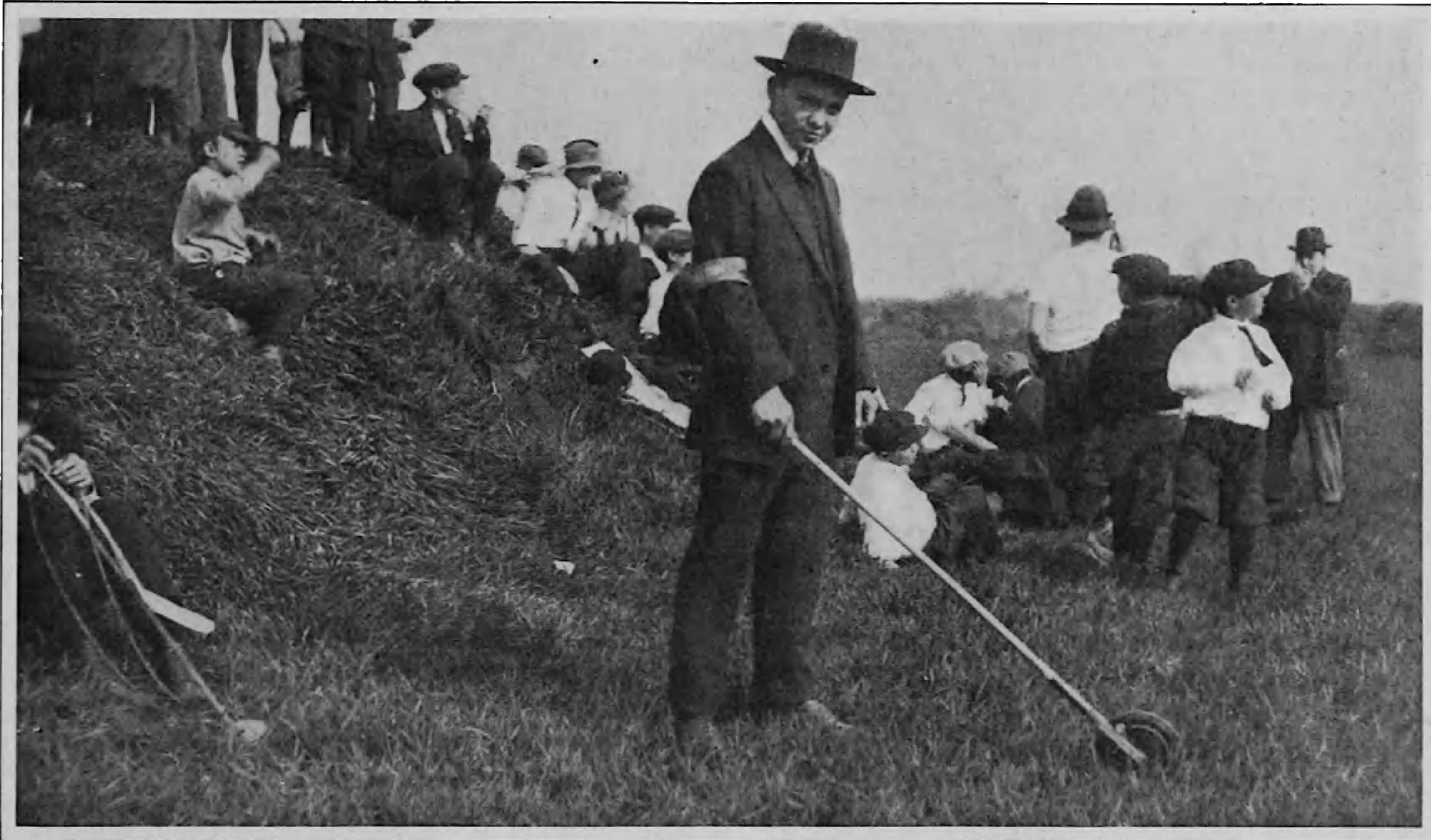
THE MEASURING DEVICE EQUIPPED WITH A CYCLOMETER.
