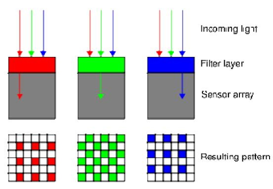
Bayer pattern on CCD sensor showing only the constituant colors passing thru.
