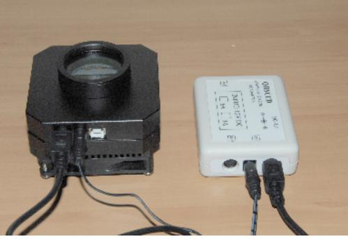
The USB socket accepts only USB2.0 interface and cables, as the camera operates at very high speeds and requires the right type of interface and cables
