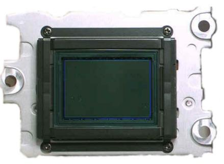
The CCD image sensors can be implemented in several different architectures. The most common are full-frame, frame-transfer and interline. The distinguishing characteristic of each of these architectures is their approach to the problem of shuttering.
