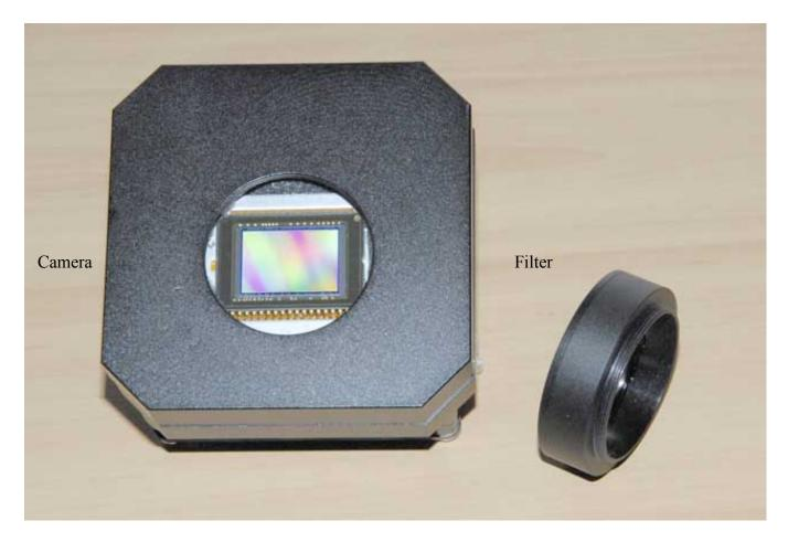
Just remove the filter like any other filter by unscrewing the nose piece anticlockwise
