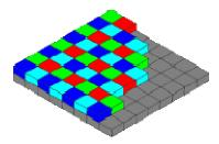
An RGBE filter on a CCD
