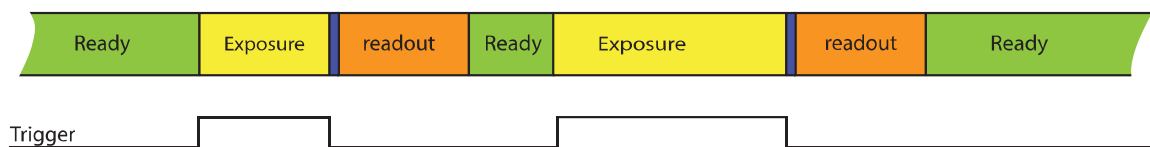
figure 4-6, Exposure defined by trigger pulse length
