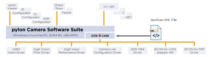
The architecture of the pylon Camera Software Suite is based on GenlCam Technology, which offers you easy access to the newest camera models and the latest features. Changes to an existing camera device in your application essentially become a plug-and-play process.
