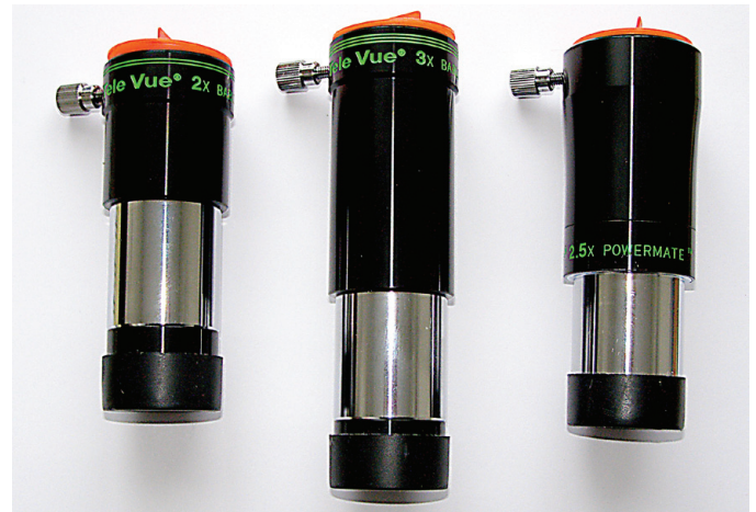
Figure 1 — Magnification amplifiers: a Barlow lens and two PowerMates™ (all illustrations by the author).
