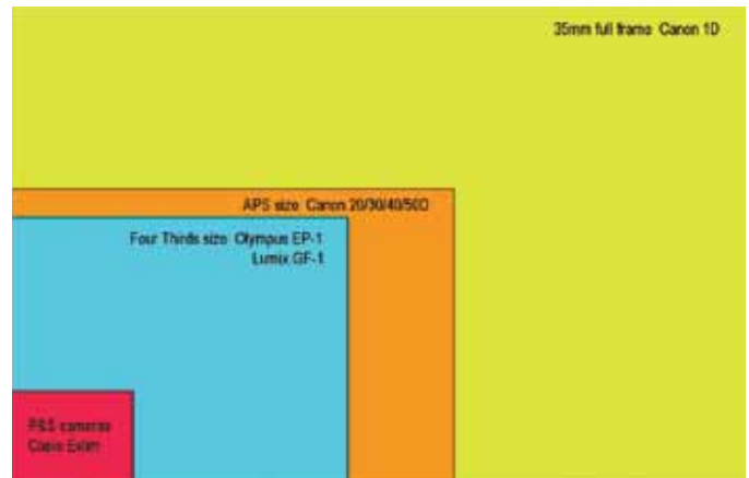
Figure 2 — Relative sizes of the sensors discussed in the text.
