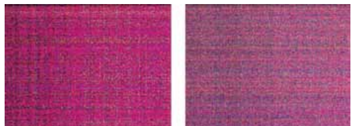
Figure 4 — Horizontal and vertical banding in the EP1 sensor.
