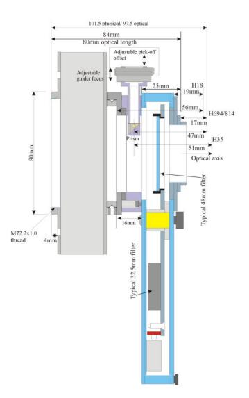
The following drawings indicate some of the options for connecting the SX-AO-USB to the guide camera and computer. The first one will be the most commonly used configuration, if you have a Lodestar X2/PRO and Trius series camera.
