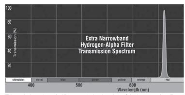
This graph shows the typical light transmission through the Orion hydrogen-alpha filter. Note that the filter only passes visible light with wavelengths between 650nm and 660nm with a full width half maximum value of approximately 7nm. All other wavelengths are essentially blocked. Transmission is greatest at 656.3nm, which is the hydrogen-alpha emission wavelength.
