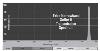
This graph shows the typical light transmission through the Orion S-II filter. Note that the filter only passes visible light with wavelengths between 660nm and 685nm with a full width half maximum value of approximately 7nm. All other wavelengths are essentially blocked. Transmission is greatest at 672.4nm, which is the S-II emission wavelength.
