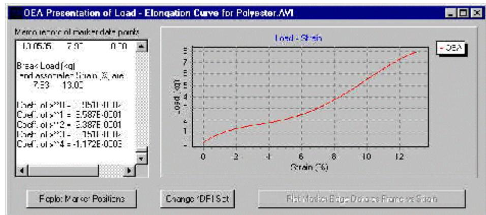
Tabulated strain, load & modulus data from individual frames. Plus test output curve, with numeric break point data and 4<sup>th</sup> order polynomial fit
