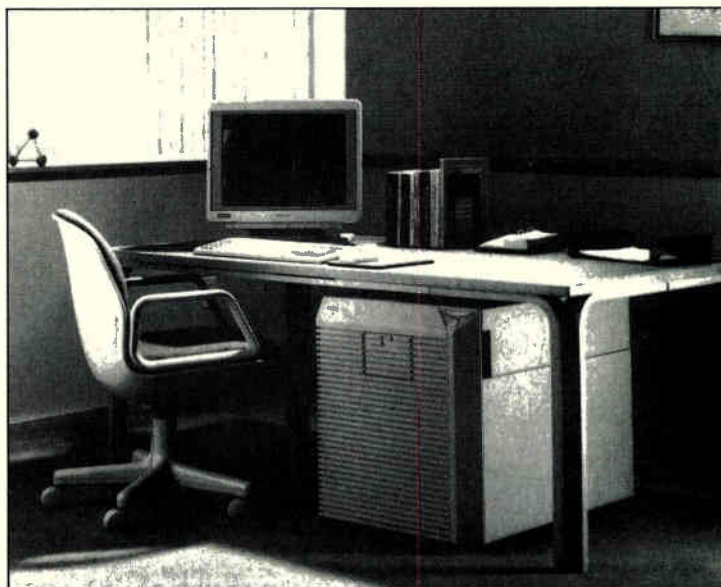
The Apollo series 10000 single-user supercomputer, which implements a RISC architecture called Prism, fits handily upon and under a desk.
