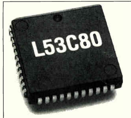
The L53C80 handles 4-Mbyte/s transfers without glitches or ground bounce.
