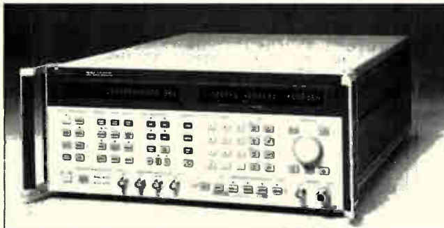
PERFORMER. HP's 8645A operates from 250 kHz to 2.06 GHz and can change frequency every 15 \mu s with an accuracy of 1 Hz per MHz.
