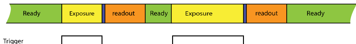
figure 4-6, Exposure defined by trigger pulse length
