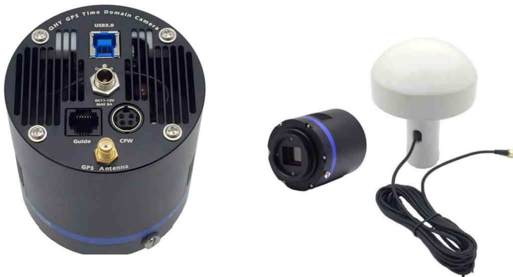
Figure 1. QHY-174M GPS CMOS camera (left) and view of the camera with GPS antenna (right)
